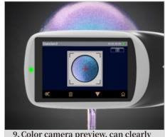
9. Color camera preview, can clearly observe the measured area Built-in color camera positioning, can accurately judge the object measured position, and improve the measurement efficiency and accuracy
